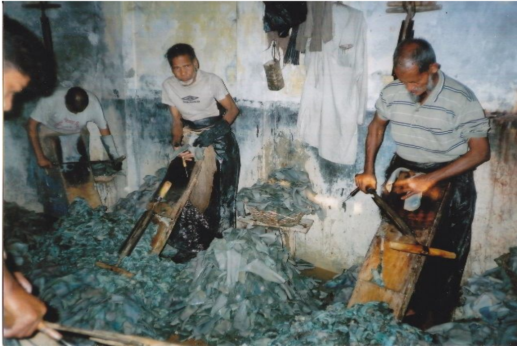
Photograph -4: Workers are removing fleshing from the pelt in M/S. Javed tannery at Hazaribagh
