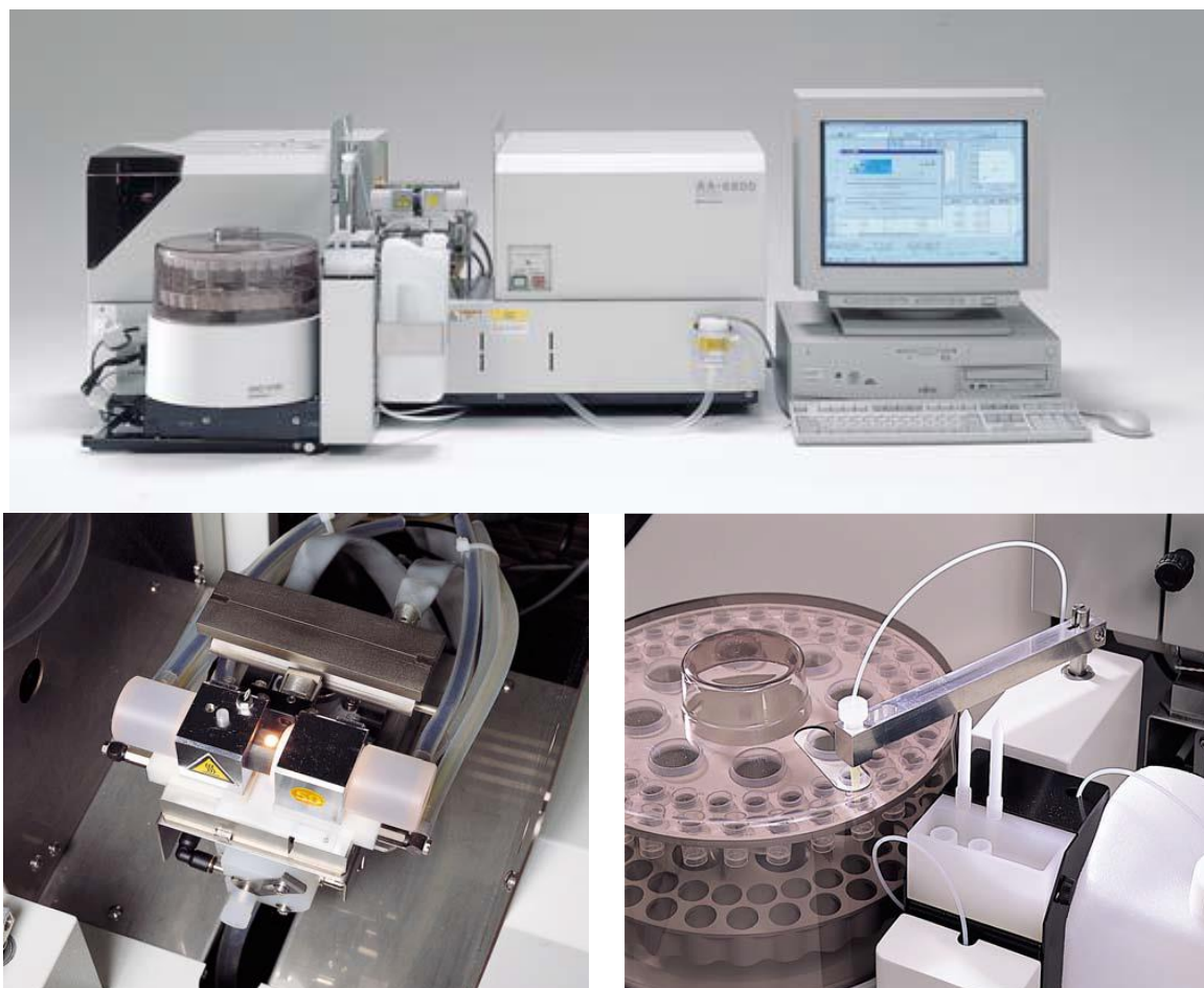
Figure 2.2 : Graphite Furnace - Atomic Absorption Spectroscopy (GF-AAS)
