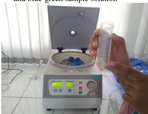
C: Precipitate collected by centrifugation
